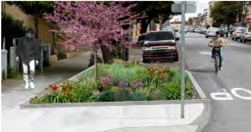
Bioretention curb extension or bulb-outs enlarge the sidewalk to incorporate the parking lane, which increases the pedestrian zone at strategic locations. This can be implemented at corners and mid block. Curb extensions enhance the safety by increasing pedestrian visibility while providing additional space for stormwater management.
